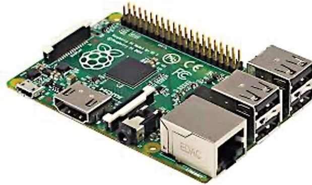
Figure 1.2: Raspberry Pi 3, Model B+, a popular single board computer
