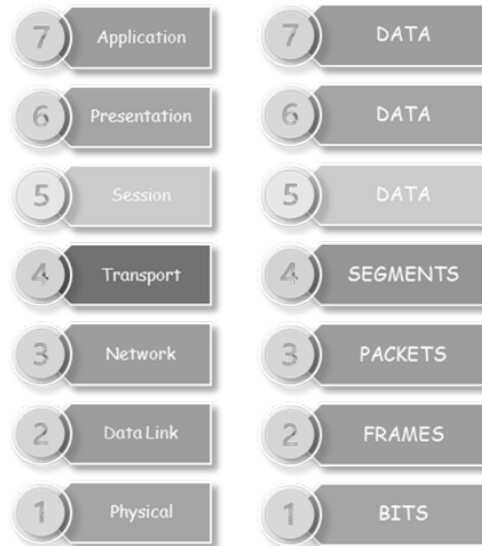
Figure 1.1: OSI model layers
